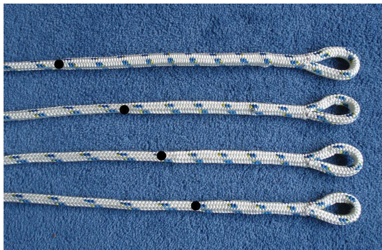
Figure 6: Completed splices with four different internal geometries. The end of each splice is indicated by a dot.
