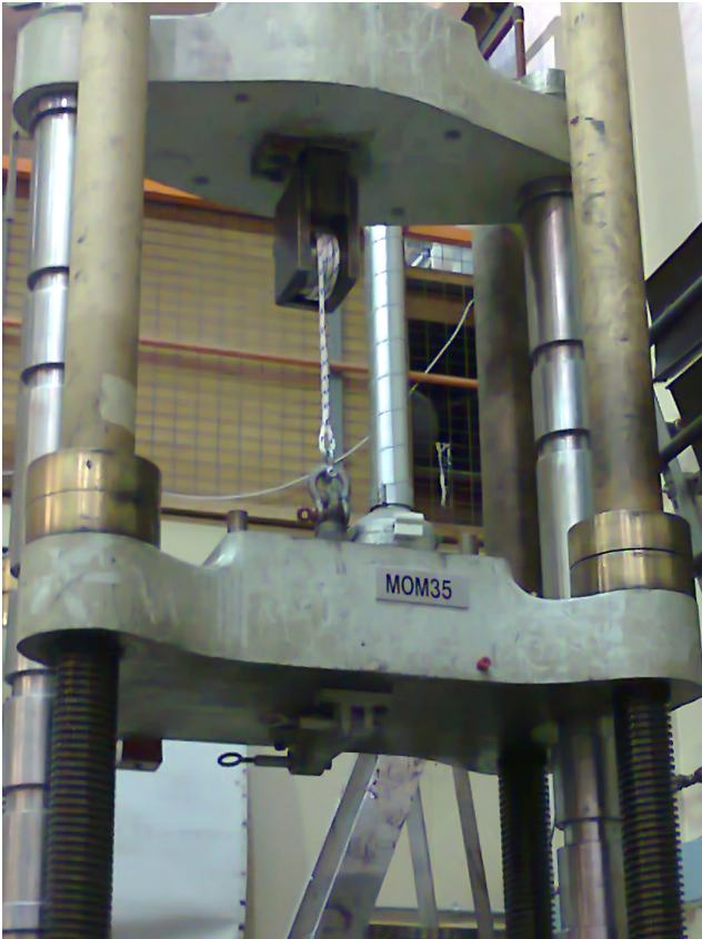
Figure 7: Setup of the Tinius Olsen tensile test machine.
