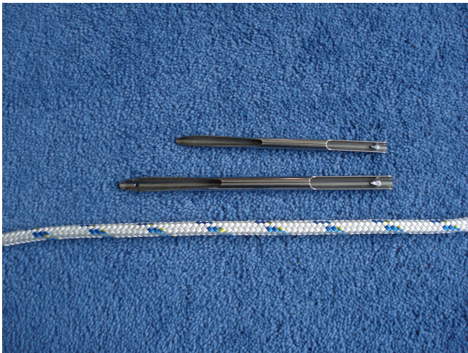
Figure 3: Swedish fids and 8mm rope. Two relative sizes of fids are generally used - the smaller for use with the rope core, the larger fid for the cover.
