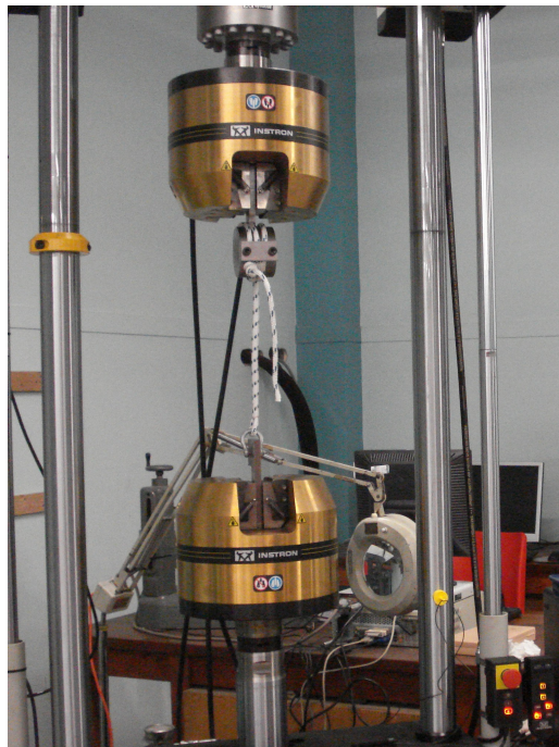
Figure 9: Setup of the Instron fatigue testing
