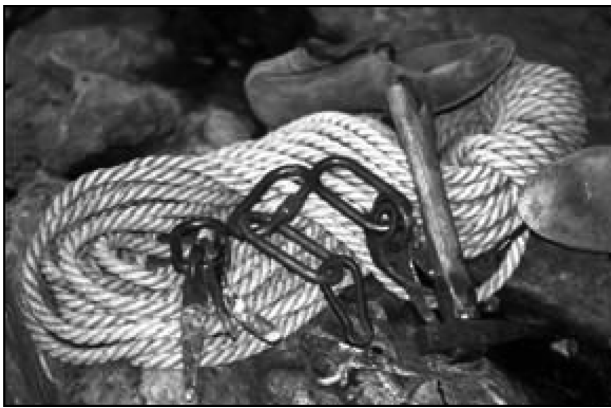
Fig. 5 Example of a hawser-laid hemp rope from the 1950s, after Schubert [19]
