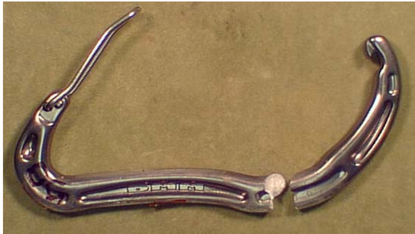
Figure 7.3: DMM deformation after Open Gate Loading
