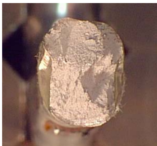
Figure 7.4: Brittle Fracture for Open DMM Karabiner
