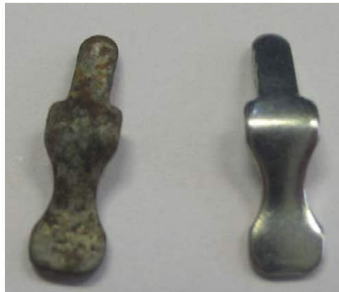
Figure 11: Comparison of spring retaining clips from sea water karabiner (left) and from new karabiner (right)
