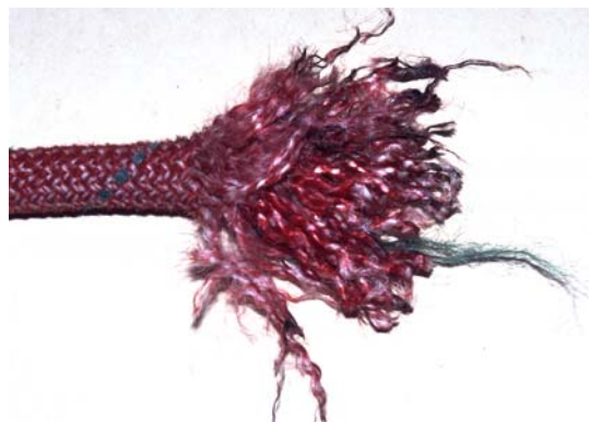
Figure 5: The broken rope during abseiling, photo by P. Schubert
