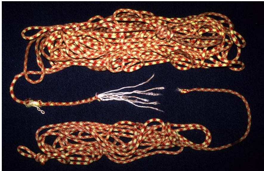
Figure 6: A rope failure by a fall over a sharp rock edge, photo by P. Schubert
