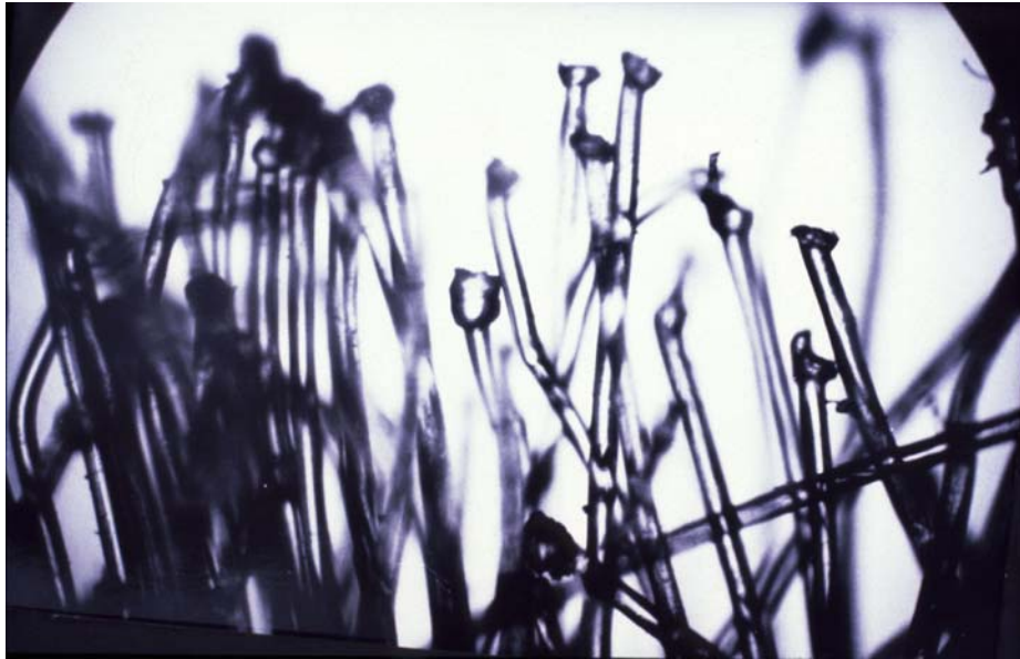
Figure 10: Filaments of a rope failure due to being cut by a knife, photo by P. Schubert
