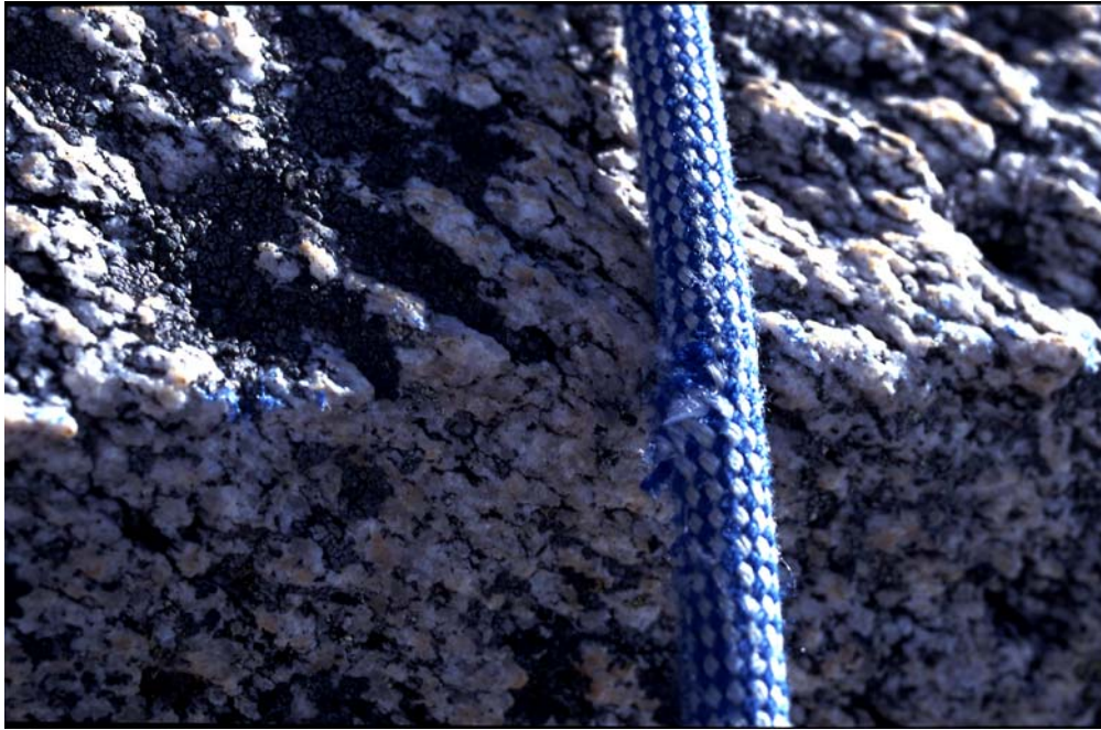
Figure 12: No rope failure, only the sheath was damaged a little bit, photo by P. Schubert
