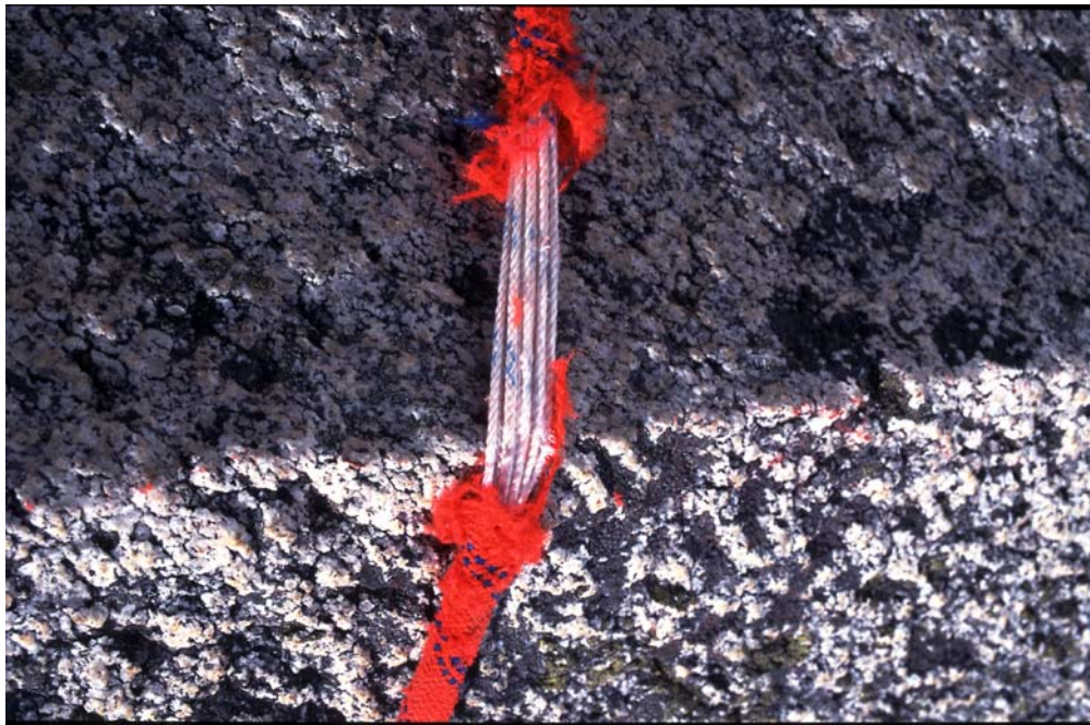
Figure 13: The thirty-nine-year-old rope: No-complete rope failure, only the sheath broke completely, photo by P. Schubert
