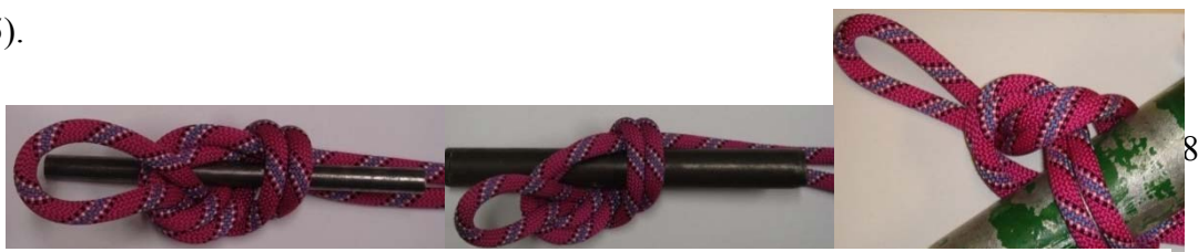
Figure 5:- Figure of eight loop with from left to right 12.5, 25 and 50mm rod inserted
