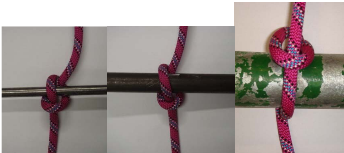
Figure 4:- Overhand knot with from left to right 12.5, 25 and 50mm rod inserted
