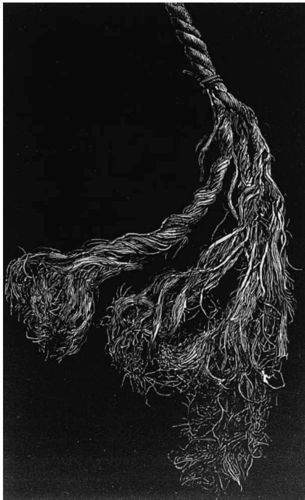
Fig. 1 Rope broken in the Matterhorn accident (Whymper, 1871).
