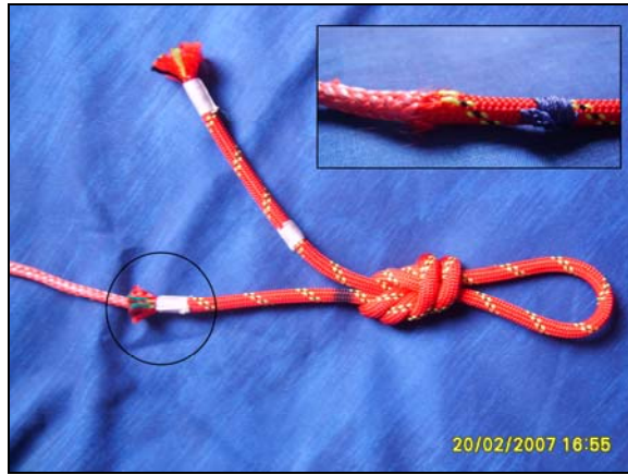
Figure 3: Specimen without tucked sheath (main picture), with a tucked sheath shown in inset
