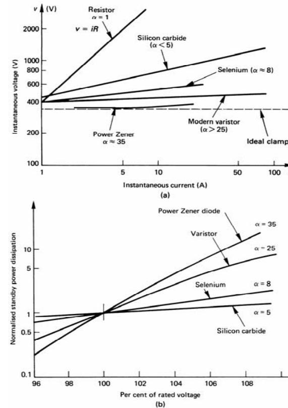
Figure 10.18. (a) The  $I$ - $V$  characteristics of four transient voltage suppressor devices, with resistance characteristics for reference and (b) standby power dissipation characteristics showing the higher the alpha the lower the standby power dissipation.
