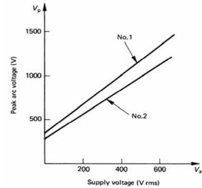
Figure 10.15. Typical peak arc voltage for two different fuse-link types.
