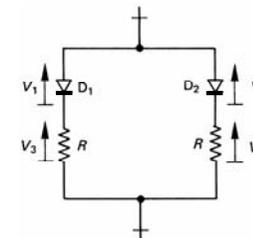
Figure 10.7. Forced current sharing network for parallel connected devices.
