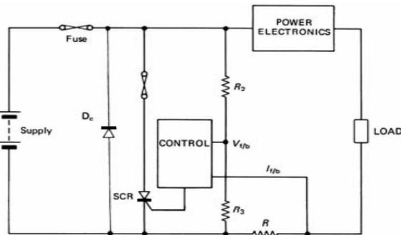
Figure 10.20. An SCR crowbar for overvoltage and over-current protection.
