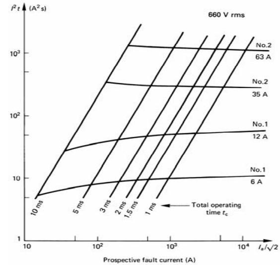
Figure 10.16. Total let-through current for total fuse-link operating times of less than 10 ms and at 660 V rms.
