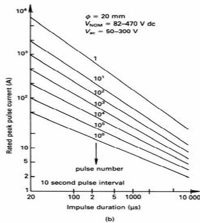
Figure 10.19. Pulse lifetime ratings for a Zinc oxide varistor: (a) lifetime for fixed 10/100 $\mu$ s pulses and (b) lifetime number for variable-duration square-wave pulses.
