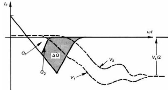
Figure 10.4. Reverse recovery current and voltage for two mismatched series connected diodes.
