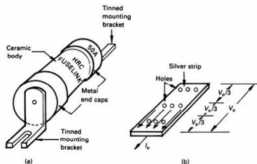
Figure 10.10. The current fuse link: (a) a 50 A 660 V ac fuse link and (b) a silver fuse link element.
