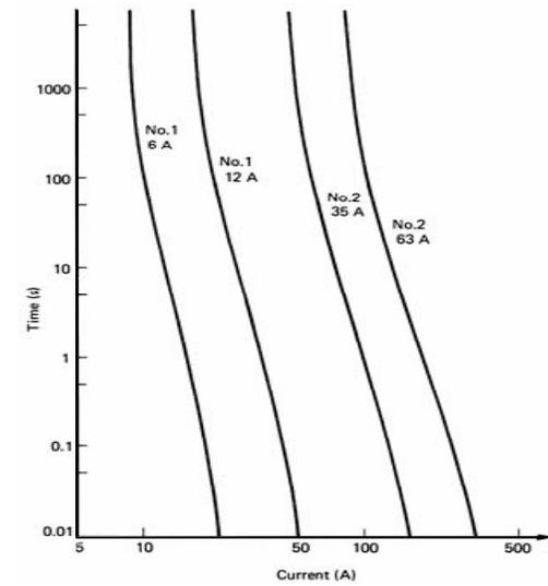
Figure 10.12. Fuse-link time-current characteristics for four fuses and symmetrical sinusoidal 50 Hz currents.
