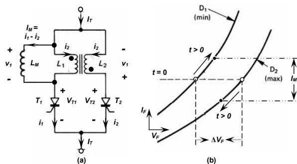
Figure 10.9. External forced current sharing network using cross-coupled reactors: (a) circuit for two devices and (b)  $I$ - $V$  operating points.
