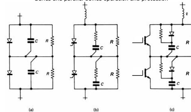
Figure 10.5. Transient and steady-state voltage sharing circuits for series connected: (a) diodes; (b) thyristors; and (c) igbt transistors.
