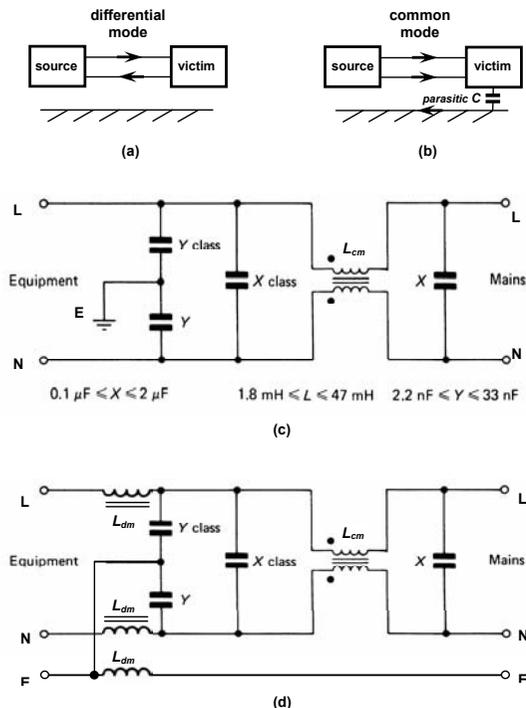
Figure 10.21. Common mode and differential mode mains supply noise filtering: (a) differential mode noise paths; (b) common mode noise paths; (c) simple L-C mains filter; and (d) high specification mains filter.
