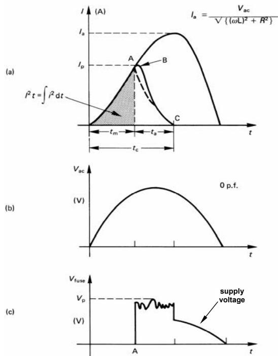
Figure 10.11. Parameters of a fuse link operating: (a) current waveforms; (b) supply voltage; and (c) fuse arcing voltage.
