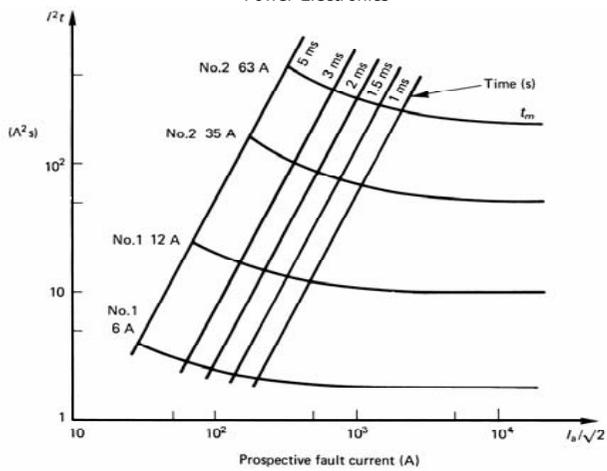
Figure 10.13. Pre-arcing  $I^2t$  characteristics of four fuse links.
