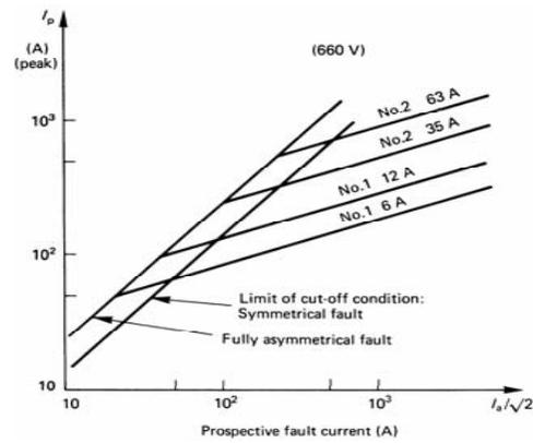
Figure 10.14. Fuse-link cut-off characteristics at 660 V rms.
