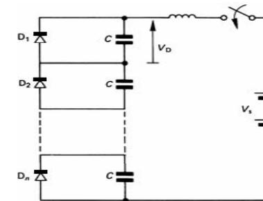
Figure 10.3. A series diode string with shunting capacitance for transient reverse blocking voltage sharing.
