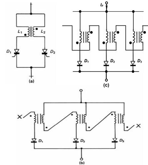
Figure 10.8. External forced current sharing network using cross-coupled reactors: (a) for two devices; and (b) and (c) for many devices.
