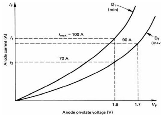
Figure 10.6. Forward conduction characteristics of two unmatched devices.
