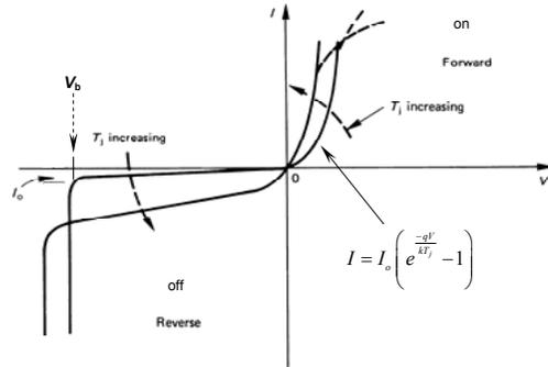
Figure 2.2. Typical I-V static characteristics of a silicon pn junction diode, and the effects of junction temperature,  $T_j$ .
