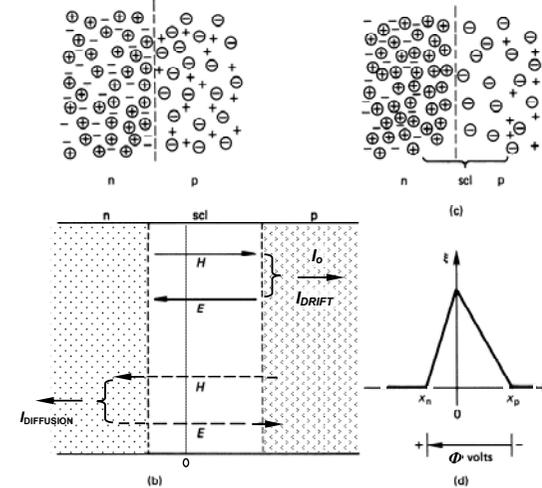
Figure 2.1. The step junction. (a) The junction if carriers did not diffuse: ⊕ ionised donors, ⊖ ionised acceptors, + holes and - electrons; (b) electron and hole movements: ---- diffusion flows, ——— drift flows; (c) equilibrium distribution of ionised impurities and free carriers; and (d) scl electric field and voltage.
