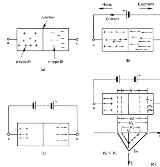
Figure 2.3. (a) Schematic of a pn junction; (b) with forward applied voltage; (c) with reverse applied voltage; and (d) electric field and scl change with increased reverse applied voltage.
