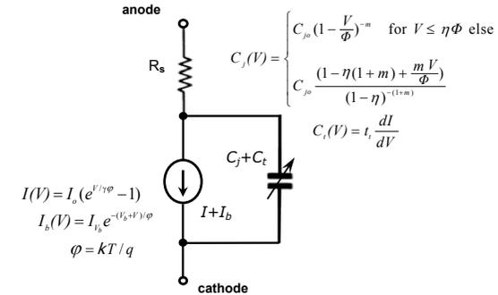
Figure 2.5. PSpice transient analysis circuit model of the pn junction diode.
