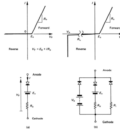
Figure 2.4. Piecewise-linear approximations of junction diode characteristics: (a) ideal diode with an offset voltage and resistance to account for slope in the forward characteristic and (b) model including reverse bias characteristics.
