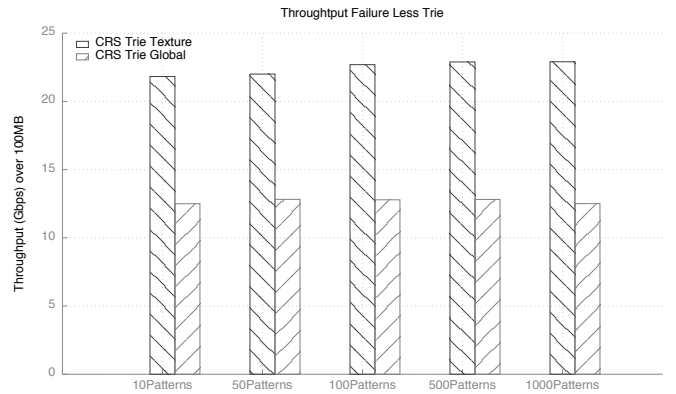
Figure 6. Throughput Comparison Between Global Memory and Texture Memory
