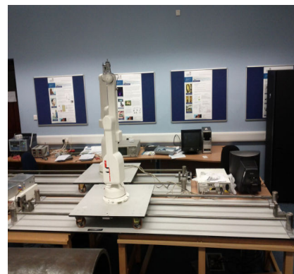
Figure 4. Robotic arm mounted on track
