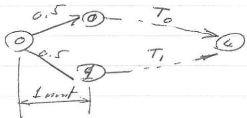
$$\begin{aligned} T_0 &= 0.5(1+T_0) + 0.5(1+T_1) \\ &= 1 + 0.5T_0 + 0.5T_1 \\ T_0 &= 2 + T_1 \end{aligned} \quad (1)$$
