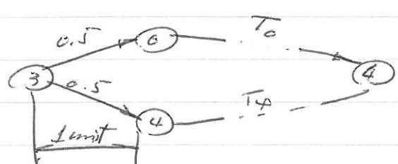
$$\begin{aligned} T_3 &= 0.5(1+T_0) + 0.5(1+T_4) \\ &= 1 + 0.5T_0 \end{aligned} \quad (4)$$
