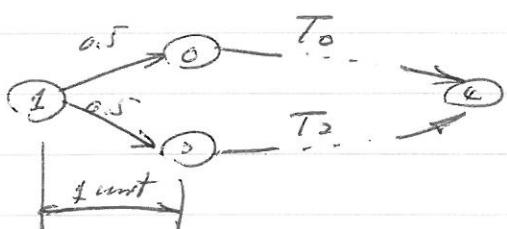
$$\begin{aligned} T_1 &= 0.5(1+T_0) + 0.5(1+T_2) \\ &= 1 + 0.5T_0 + 0.5T_2 \end{aligned} \quad (2)$$
