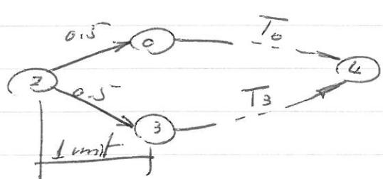
$$\begin{aligned} T_2 &= 0.5(1+T_0) + 0.5(1+T_3) \\ &= 1 + 0.5T_0 + 0.5T_3 \end{aligned} \quad (3)$$
